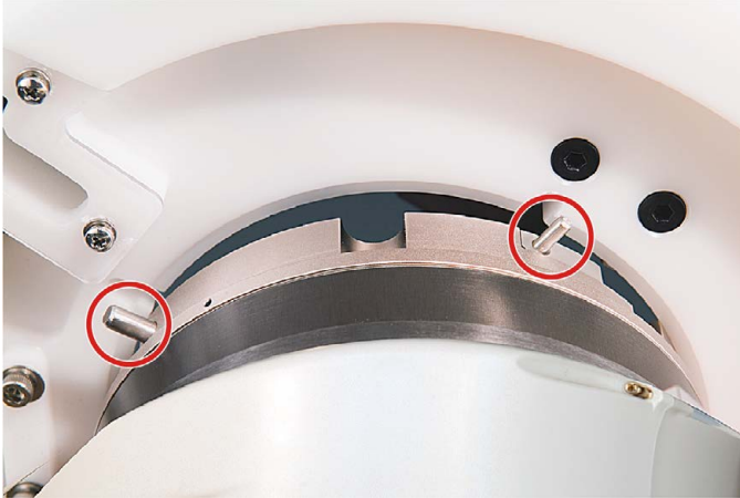
Figure 5-2: Notches on the filler aligned with the pins on the centrifuge
