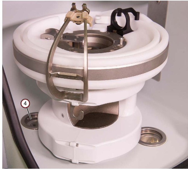
Figure 2-4: AIM system light behind the gear shroud
